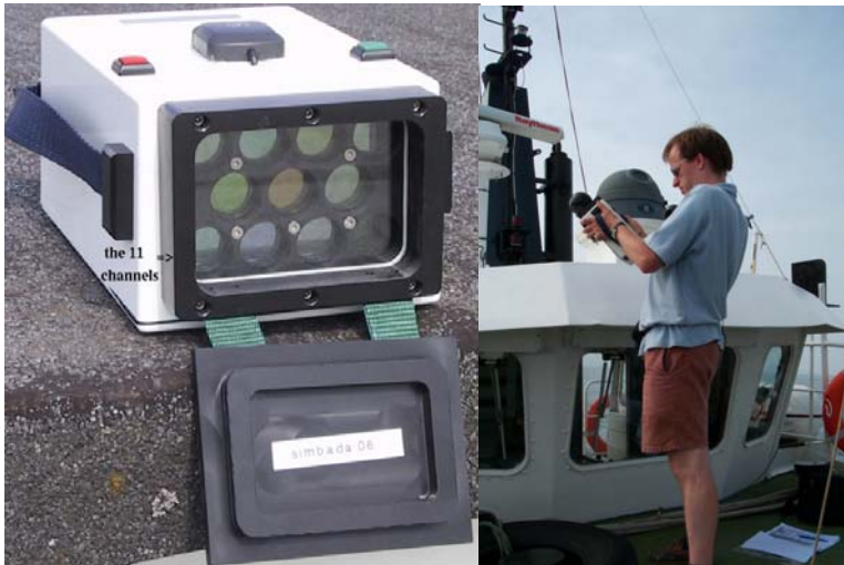
Figure 11. (left) View of SIMBADA showing foreoptics. (right) As used in sun-viewing mode.
