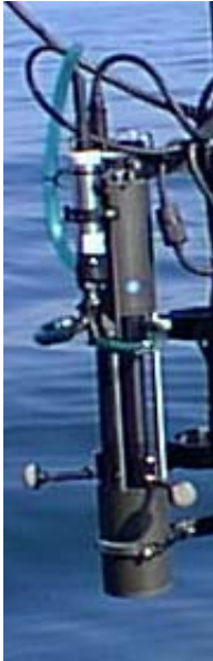
Fig. 4: AC-9 unit (WETlabs Inc, USA)
