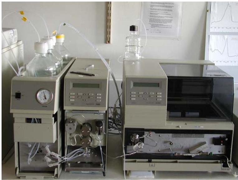
Figure 5: Diode array detector (UV6000LP) and pumping system (P4000) for High performance liquid chromatography.
