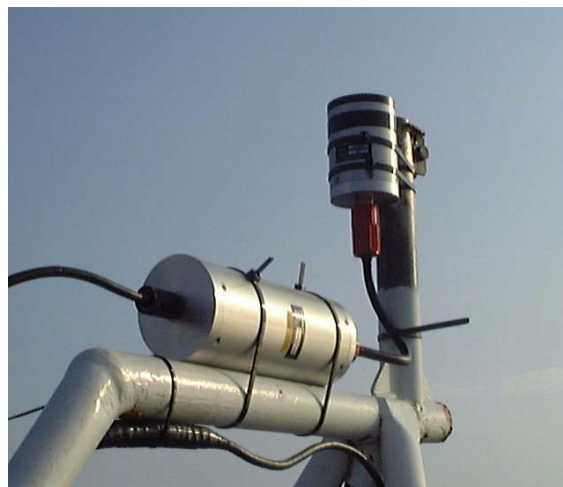
Figure 6: Satlantic sensor head for E_s(\lambda) measurements.
