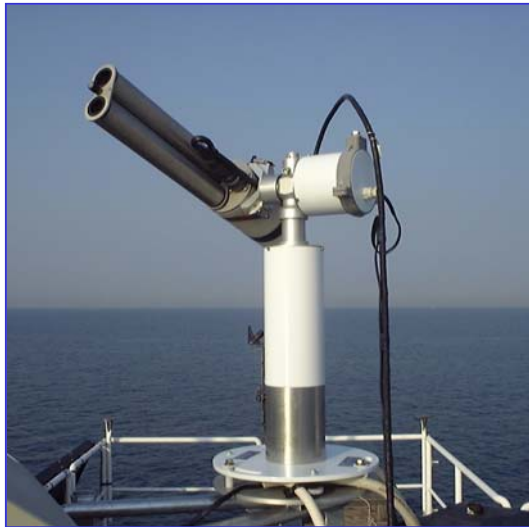
Figure 8: CE- 318 Sun photometer
