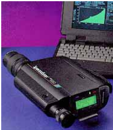
Figure 9 : PR650 instrument PR®-650/640 SpectraColorimeter™ System.
