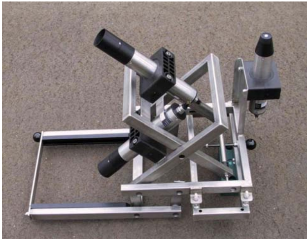
Figure 10. (left) System of two radiance and one irradiance sensor installed on steel frame. (right) As installed at prow of ship with irradiance sensor mounted separately to reduce optical interference from mast.
