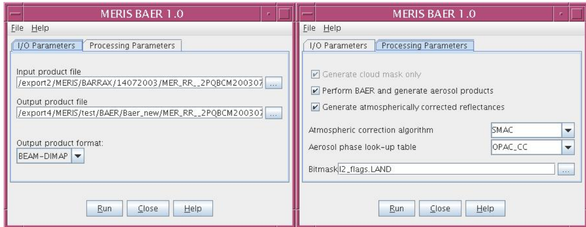
Figure 18: Integrated Baer processor panels
