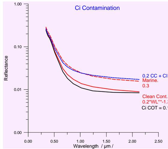
**Figure 6: Spectral TOA reflectance for clean continental aerosol model (red solid line) and a thin Ci cloud (black line) separately and their composed effect (blue line). For comparison a marine aerosol model fits with the composed conditions.**
