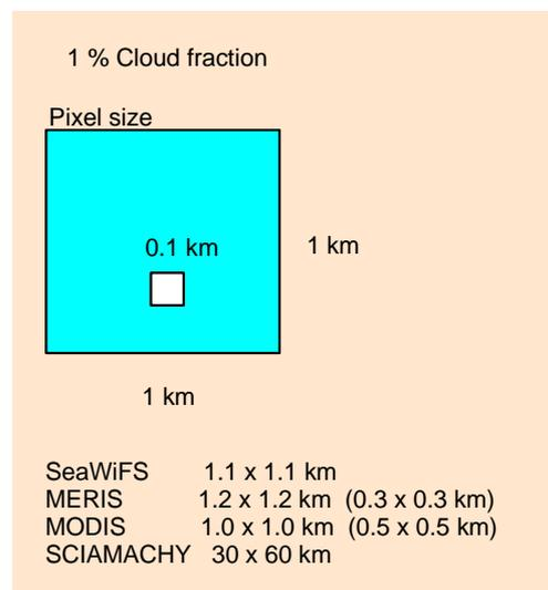
**Figure 3: Representation of a sub pixel cloud in a pixel.**
