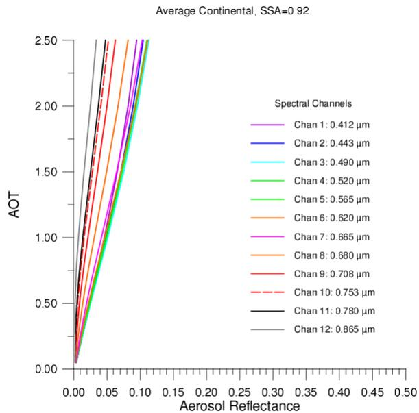
**Figure 13 LUT for case 3 with an aerosol phase function and a single scattering albedo  $\omega_0 = 0.928$  of the 'average continental' aerosol model from OPAC 3.1 Hess *et al.* (1998), for land surface conditions for the different channels of MERIS.**
