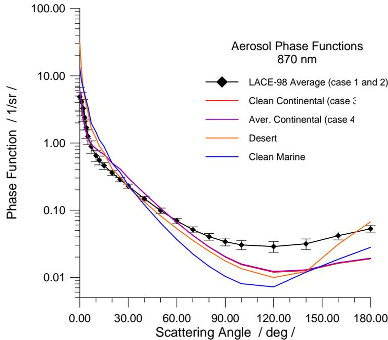
Figure 10: Aerosol phase functions of the cases used for the LUT : (a) experimental phase functions from LACE-98, cases with increased lateral scattering (thick black curves, used in case 1 ), (b) 'average continental' (case 3) and 'clean continental' (case 2) from OPAC. Two more cases are shown in the plot 'desert' from OPAC and 'clean maritime' from OPAC.
