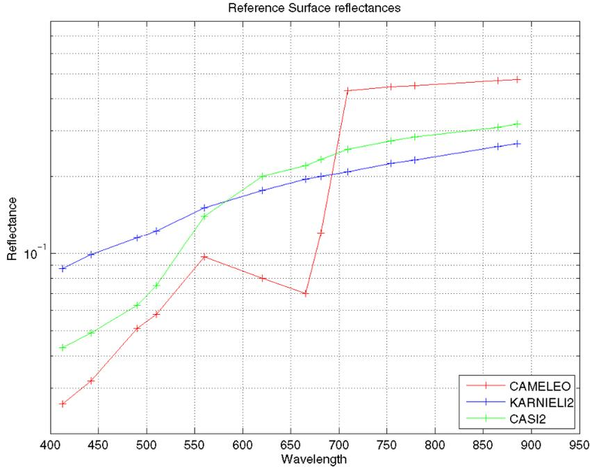
**Figure 8: Spectra used for the determination of the apparent spectral surface reflectance within the BAER approach: The ‘CASI2’ soil spectrum is taken from CASI-radiometer measurements (Olbert (1998)) and the KARNIELI2 desertic spectrum soil is taken from Baret (personal communication). The vegetation spectrum is taken from the CAMELEO database, Escadafal and Bohbot (1999).**
