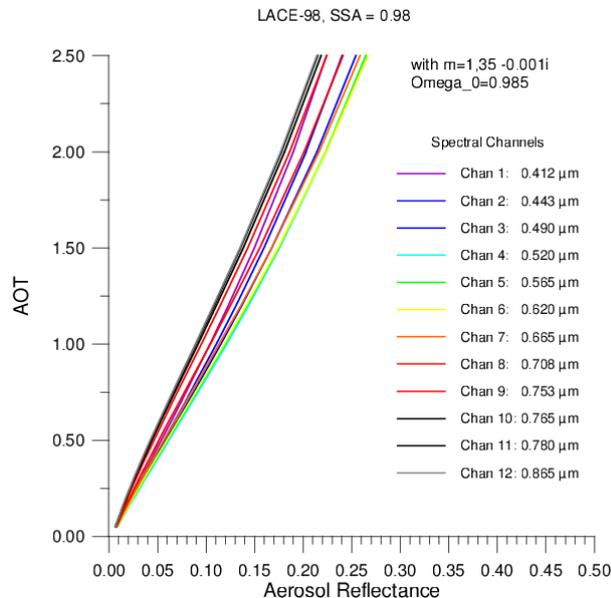
Figure 11: LUT for case 1: LACE-98 aerosol phase function and a single scattering albedo  $\omega = 0.98$ , for land surface conditions for the different channels of MERIS.
