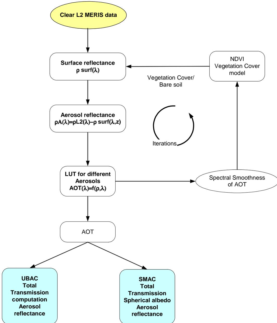
Figure 14: Scheme of the retrieval procedure for the surface reflectances over land.
