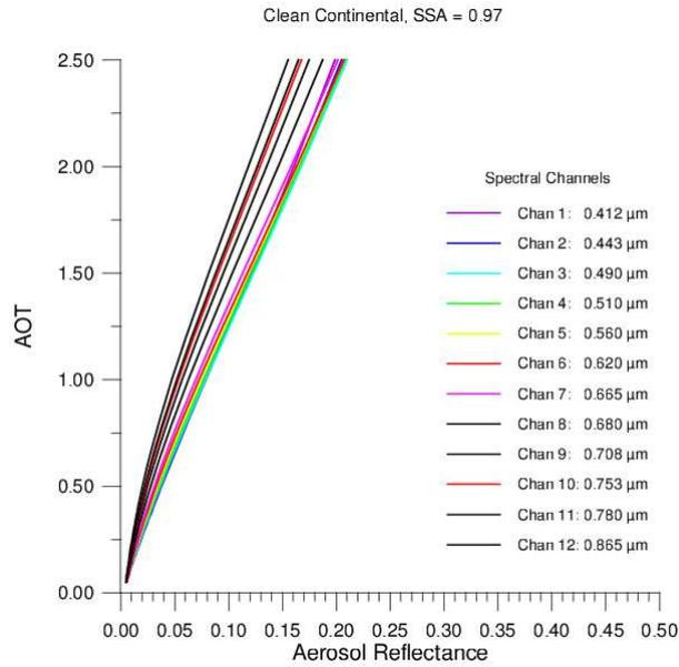
**Figure 12: LUT for case 2, using the aerosol phase function and a single scattering albedo  $\omega_0 = 0.975$  of the 'clean continental' aerosol model from OPAC 3.1 Hess *et al.* (1998), for land surface conditions for the different channels of MERIS.**
